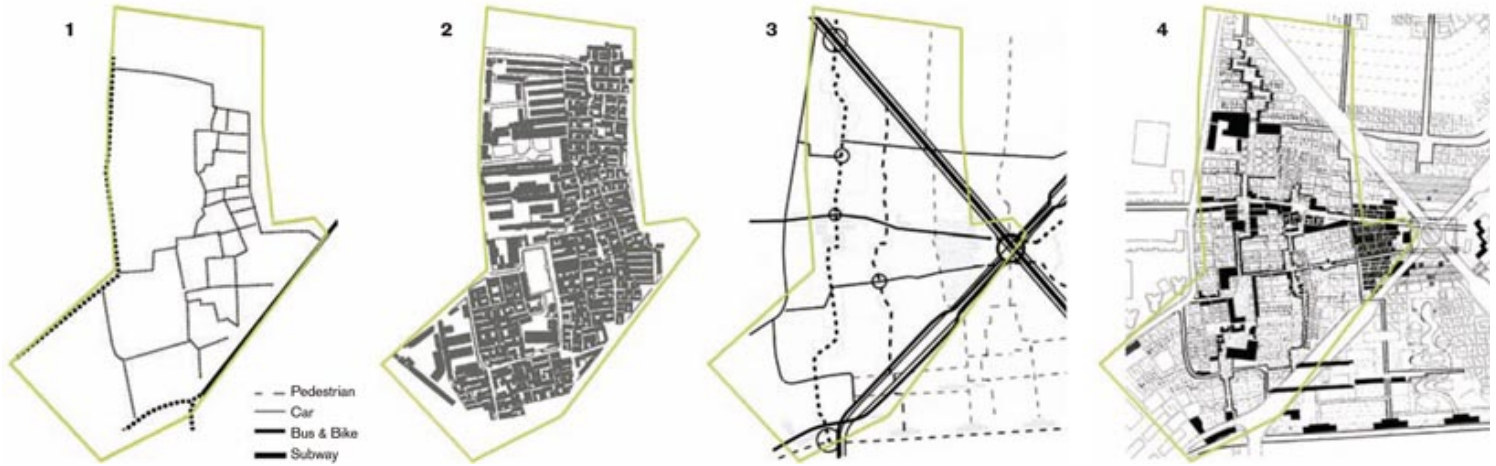
1. Existing circulation; 2. Existing textural form—reveals rice paddy configuration and irrigation canals; 3. Proposed circulation—hierarchy of primary, secondary and tertiary routes based on the farming structure; 4. Proposed textural form and civic structure—textural form is integrated into the rice paddy module while the public civic structure links the existing north-south axis with the new transport station.
