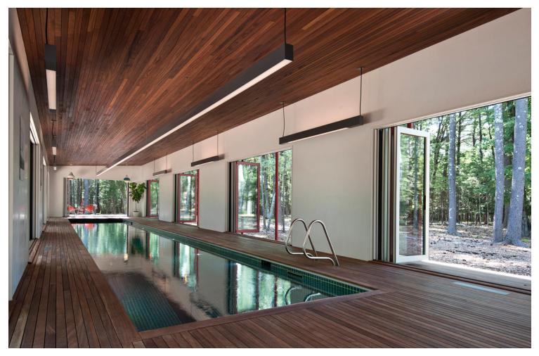
Materials were selected for their durability and beauty, and include sapele wood flooring, decks and ceilings, locally sourced limestone floors and counters, waterproof plaster walls, custom fabricated light fixtures, standing seam Galvalume roofing, and custom-milled Eastern White Pine siding and timbers, most of which was carefully harvested from the building site while leaving others towering above.
