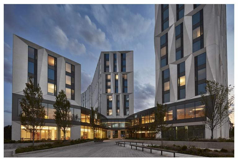
The building is scaled to its context, with the highest structure completing the urban edge of busy 55th Street, while nearby structures are more attuned to the residential neighborhood along University Avenue. Pre-cast concrete panels are used to clad the building, a contemporary facade informed by the University's gothic tradition.
