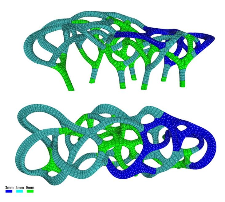
Shortly after the last pieces were riveted in place, Tampa withstood extreme wind loads from Category 4 Hurricane Michael. But the structure was devised to stand up to such weather: its 3,123 parts make up a double-layer structure, with rings forming the interior layer of the columns and stripes cross-laminating as an exterior skin to compose the branching elements.
