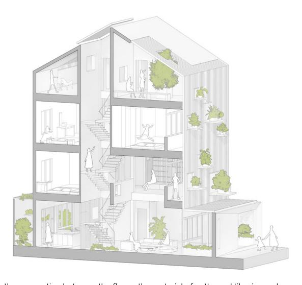
To strengthen the connection between the floors, the material of patterned tiles is used continuously from the wall of one tube to the floor adjacent to the other tube, exiting onto the façade of the house. This solution of using material blurs the space vertically and horizontally, connecting all floors in a direct and physical way.
