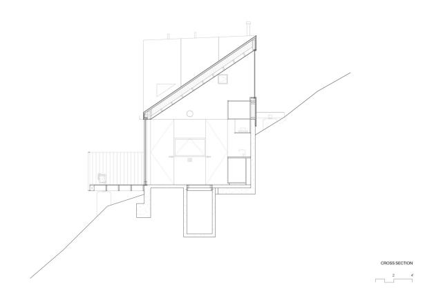
Due to the incredibly steep hillside, a deck was added on the front of the ADU to add more usable exterior space to take advantage of the mild California climate, essentially doubling the ADU's usable area. Designing for the utmost effective square feet (411 sq.ft. / 38 square meters), flexible programming was deployed: a rolling kitchen island can be moved in or outside when space or utility is needed, and a murphy bed hides in the wall during the day and folds down at night for sleeping.
