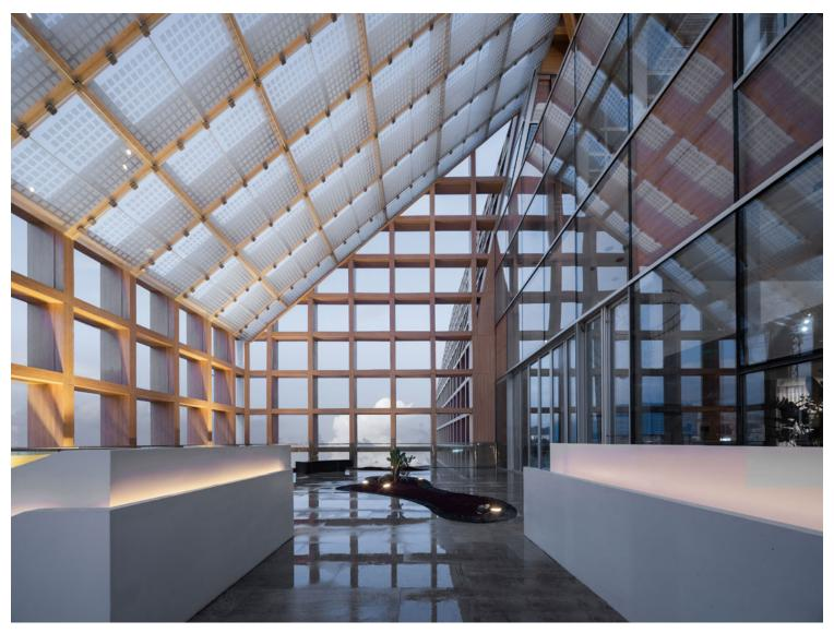
The inclined and horizontal shelf-like grid elements are fitted with gutters for drainage. Rainwater harvested here can be used for landscape irrigation across the building.
