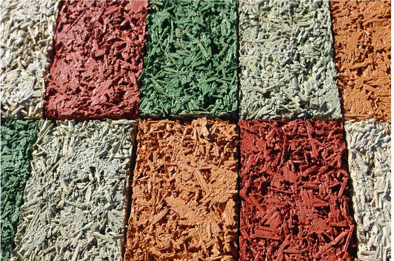
Natural and colored hemp lime concrete samples
