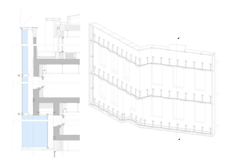
The glass panels that make up this pleated structure are supported by stainless steel rails. An anodized aluminum frame allows for natural ventilation of this double skin. The upper part of this frame, which constitutes the acroterion, is made up of removable panels that make its maintenance possible.
