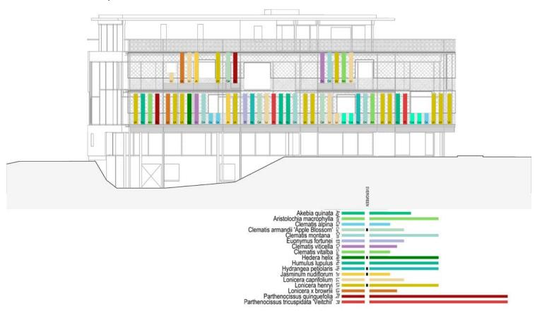
Rainwater from the roof is collected in an underground cistern and feeds the automatic irrigation system for the plants on the façade and the garden. Together with the 1,215 new plants in the open space, incorporating 73 local species, the green façade also contributes to local biodiversity, ensuring that the building is a good neighbor to its human and non-human communities.
