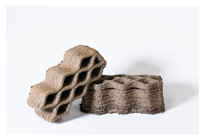
The 3D printed brick experiments using varying mineral content
