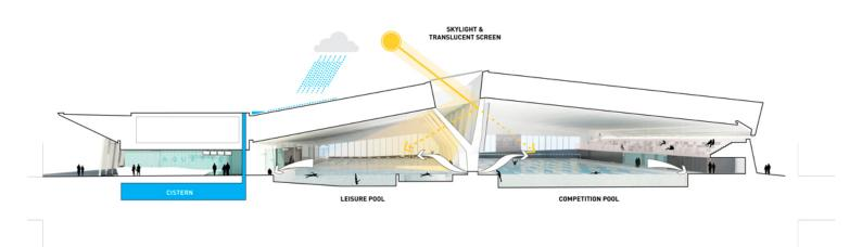
Water: A three-compartment cistern will store water from the roof and adjacent transit plaza. The water will 'top-up' evaporative loss in the basins, provide for grey water flushing, and supply a site irrigation system.
