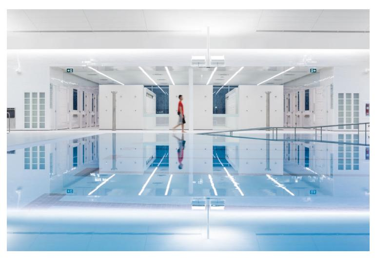
Light: The sectional split brings light deep into the centre of the natatorium plan, where it is reflected or diffused to provide the required natural lighting condition. A continuous ceramic fritted glazing band on three elevations and sensors for zoned lighting control respond to the level of natural light.
