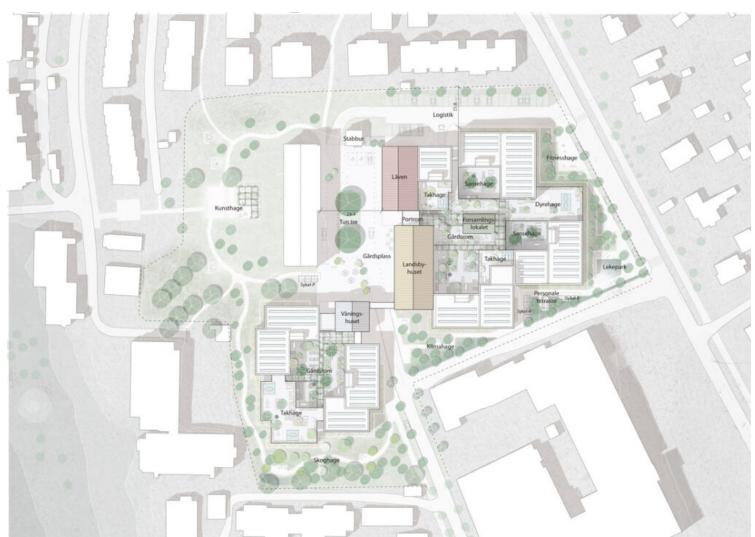
All the housing units have an outdoor access connected to the common spaces, and the layout is developed with a focus on dementia, where all the residents' rooms face the common rooms rather than a corridor. All circulation spaces are designed as loops of various sizes to enable physical movement without getting lost or running into a dead-end.
