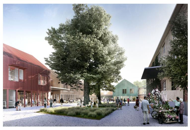
By splitting the volume into smaller units and maintaining a height of two stories, we create a complex with a human scale. Together with differentiating the buildings by color and shape, this significantly helps wayfinding for people with cognitive disabilities.
