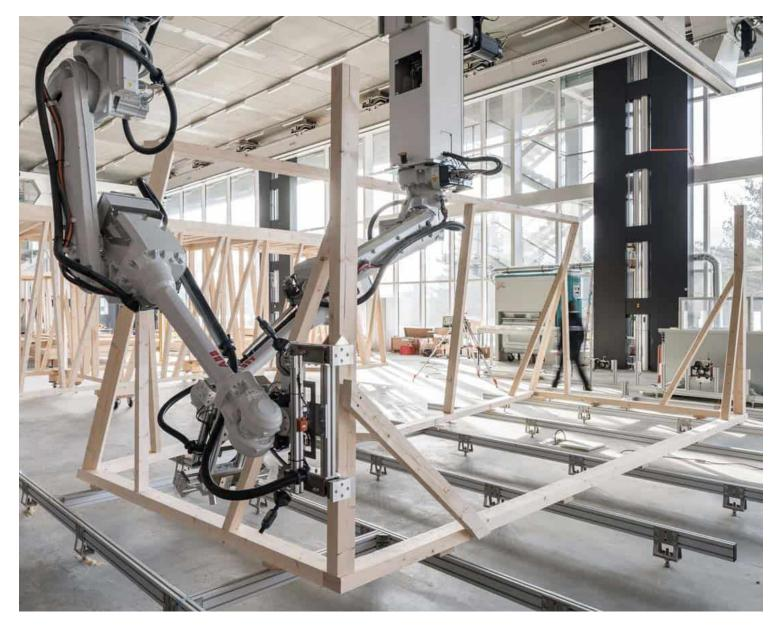
The two cooperating robots precisely position the timber beams in the spatial arrangement predefined by the computational design without colliding.
