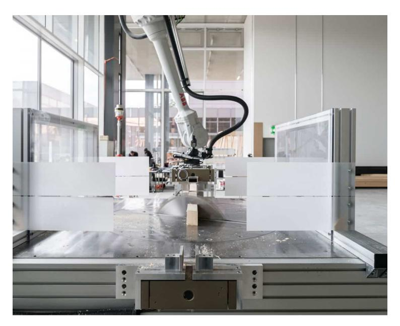
One of the robots taking a timber beam to the saw in order for it to be cut to size.
