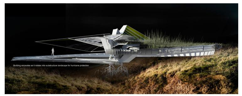
The excavated ground is pushed away, whilst the artificial island surrounding the building acts as a canopy moving water away from the building. Solar panels line the island's floor plate panels and, edged by a ring of turbines, the turntable-like design consists of sixty-four separate timber sections
