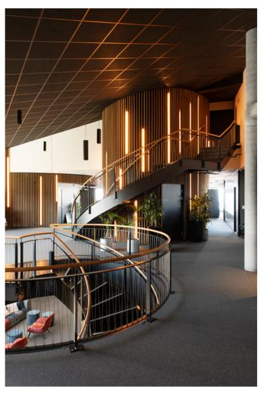
In order to reduce energy use on lighting, the building employs a concept called "liquid light", which allows the artificial light to smoothly dim up and down according to the activity and movement in the building. Taken together, these strategies allow Powerhouse Brattørkaia to consume only about half the amount of energy for lighting compared with a typical commercial office building of a similar
