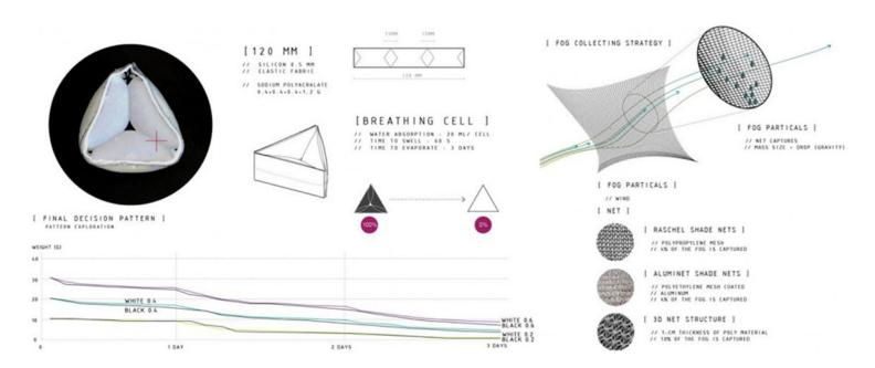
Hydromorph cell geometry and fog collection strategy. The cell is able to open and close as a result of the changes on the volume of hydromorph.
