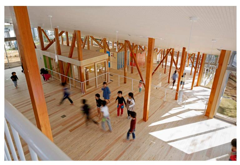
Utilizing large sliding window frames along the northern and southern faces, along with the space created by the slope, ventilation is created as a breeze draws in from the south of the structure, passes through the forest-like interior pillars making its way upwards before finally blowing out across the terrace on the northern side.
