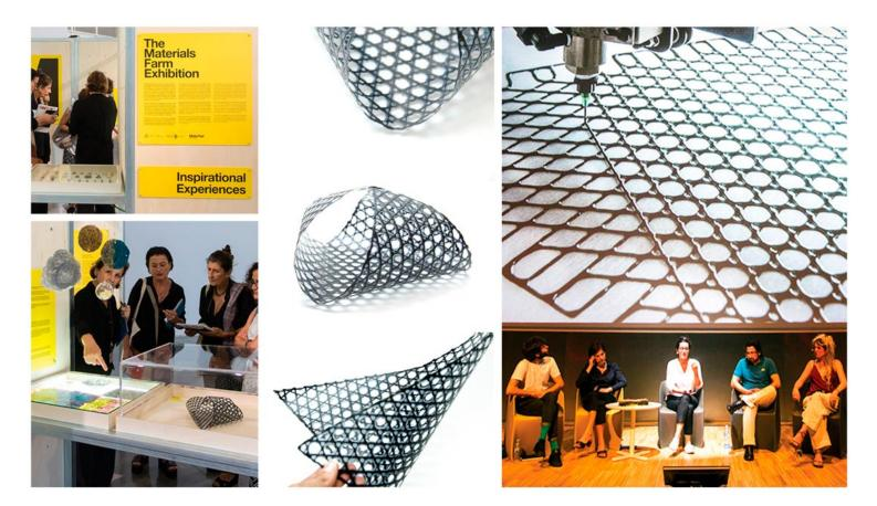
At the past "Materials Farm" exhibit at FADFest Barcelona 2017, a macro-lattice basket was 2.5D-printed out of colored silk fibroin and displays tunable flexibility for durable bending capabilities. It was developed using green chemistry and ensured ultimate biodegradation. Developed by architect Laia Mogas at the Living Materials Silklab, led by Dr. Fiorenzo Omenetto.
