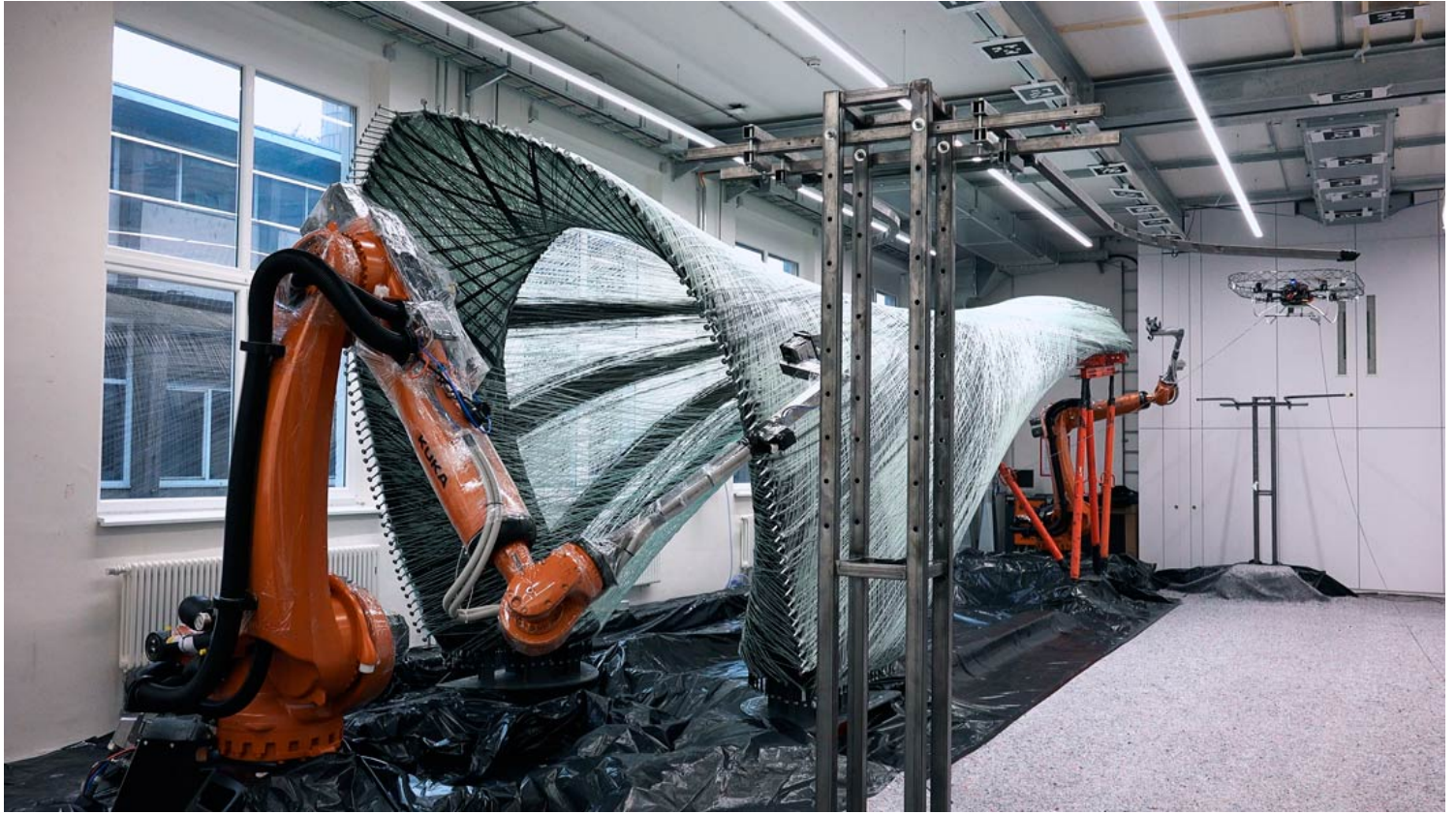
Autonomous flight of custom drone carrying a fiber between robots
