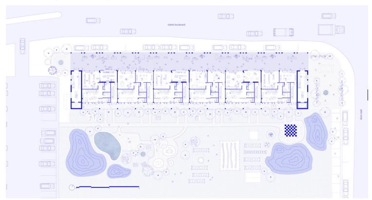
The triple-height greenhouse structure covers a shared terrace on the private side of the building, which becomes a semi-public, semi-exterior mediator in addition to being a climate strategy. While occupants remain protected from wind and precipitation, sunlight filtering in through the translucent high ceiling evokes the outdoors in a space that is comfortable and habitable year-round.
