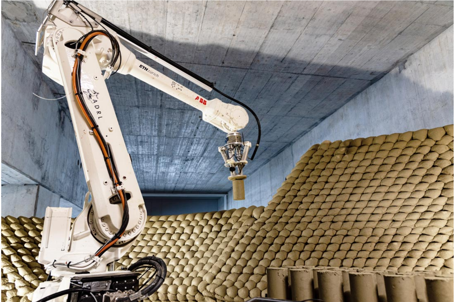
Clay Rotunda, fabrication setting with robotic arm, SE SEMUSICLAB, Bern 2020-2021 © Gramazio Kohler Research, ETH Zürich. Photo: Indra Santosa
