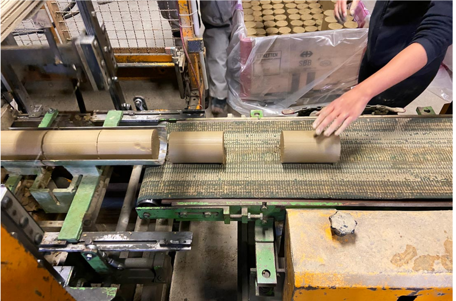
Clay Rotunda, fabrication of the soft-bricks at Brauchli Ziegelei AG, 2020-2021 © Gramazio Kohler Research, ETH Zürich. Photo: Coralie Ming
