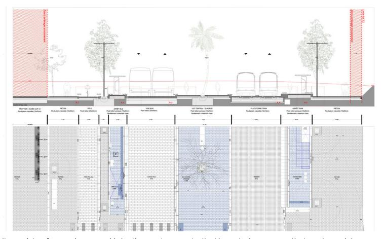
It consists of an underground irrigation system controlled by exterior sensors that cool special breathable pavers, manufactured experimentally using mollusc shells.
