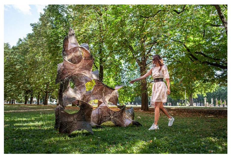
The Mock-up is 2 m high, consists of 14 modules and weighs only 20 kg. The identical modules were assembled into different foam-like lightweight compositions. The modules were fabricated by digitally tailoring natural flax fibers into specific 2D patterns following optimized structural and parametric geometrical deviations. These were later formed using a vacuum-assisted molding process into the final 3D shapes.
