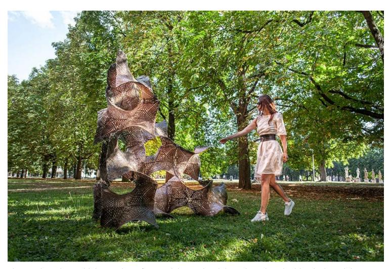
The Mock-up is 2 m high, consists of 14 modules and weighs only 20 kg. The identical modules were assembled into different foam-like lightweight compositions. The modules were fabricated by digitally tailoring natural flax fibers into specific 2D patterns following optimized structural and parametric geometrical deviations. These were later formed using a vacuum-assisted molding process into the final 3D shapes.
