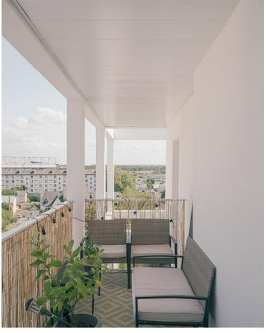
The buildings are designed on a working grid system adhering to a rigorous structural rationality. The upper floor façades rise on a post-and-beam matrix in white-painted concrete with regular setbacks to allow for different uses, terrasses or storage areas. This matrix establishes the visual identity of the new buildings, casting shadows over the outdoor spaces, providing supports for hanging sunshades or creating the privacy needed for communal living.
