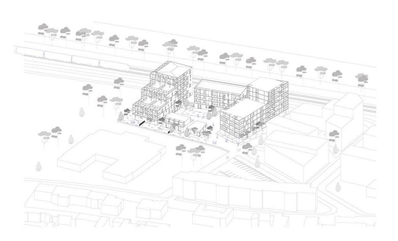
The tiered design of Building A follows the basic project grid and helps to create the most user-friendly outside spaces. The stepped volumetric approach also provides the necessary visual protection for the adjoining school to the south, limiting the views over the playground.
