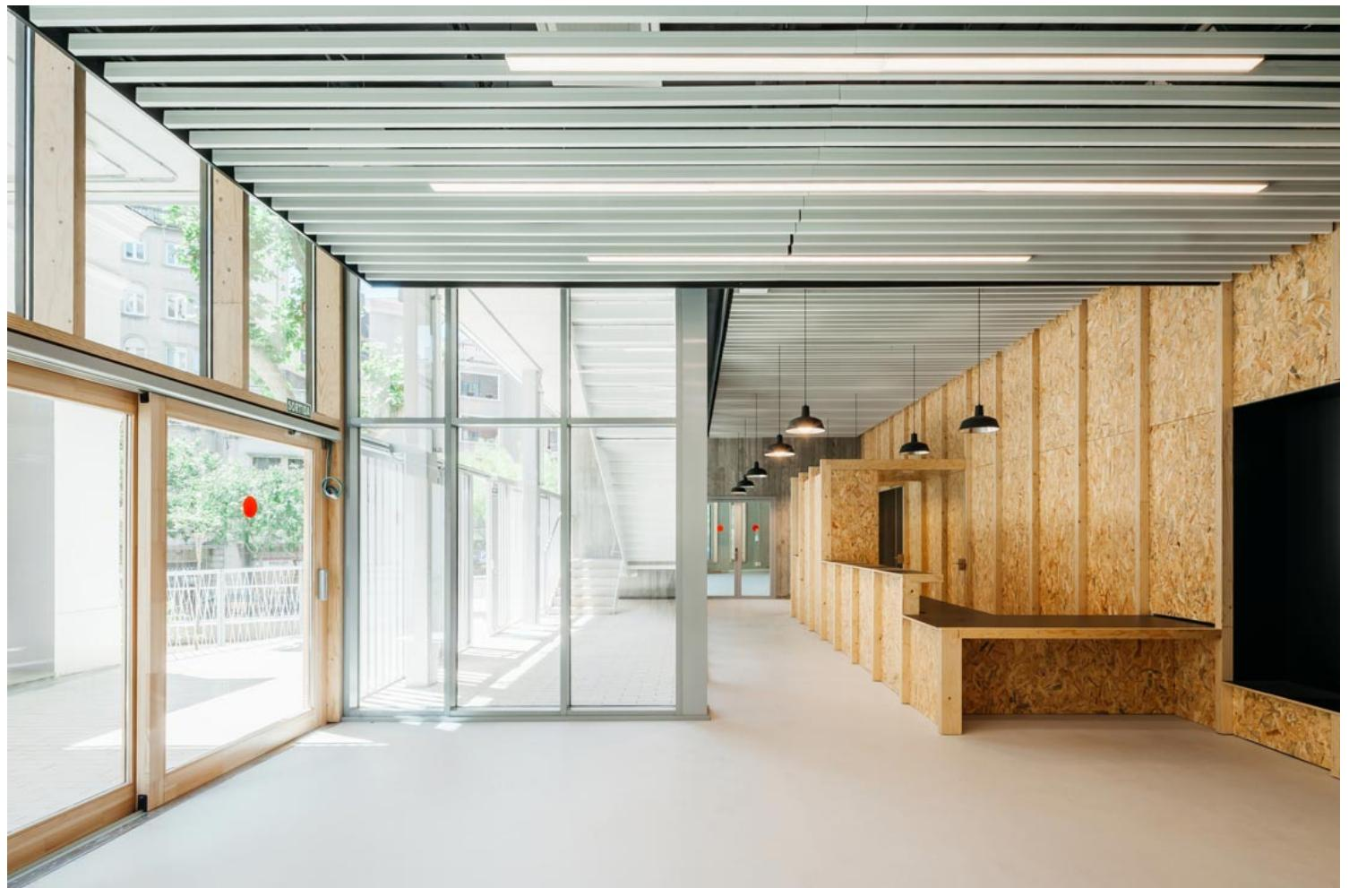
The building is notable for its intense use of materials with a low environmental impact that are recycled and renewable. This includes wooden structures and wooden carpentry, wood-aluminium curtain walls or hemp fibre isolation panels.
