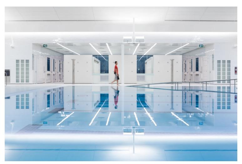
Light: The sectional split brings light deep into the centre of the natatorium plan, where it is reflected or diffused to provide the required natural lighting condition. A continuous ceramic fritted glazing band on three elevations and sensors for zoned lighting control respond to the level of natural light.
