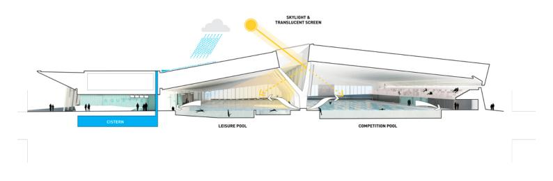
Water: A three-compartment cistern will store water from the roof and adjacent transit plaza. The water will 'top-up' evaporative loss in the basins, provide for grey water flushing, and supply a site irrigation system.
