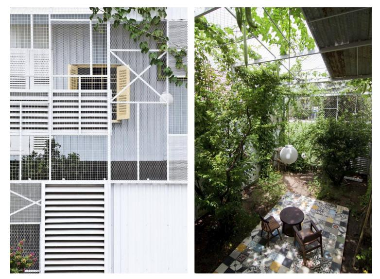
Given the budget constraints, a light structure in steel and sheet metal was used instead of bricks and concrete as usual. Moreover, recycled furniture that has been abandoned but is still in good condition, is used as an appropriate solution for most parts of the house. This not only reduces construction costs, but also gives the house a distinctive look: the beauty or serenity of old items that comes with age.
