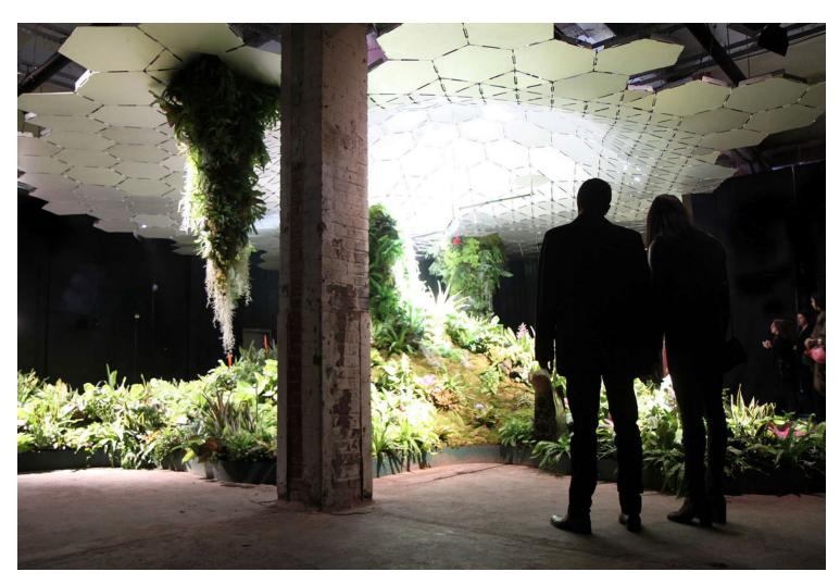
James Ramsey, his team at Raad Studio, and the Korea-based technology company Sunportal designed and installed optical devices which capture and concentrate natural sunlight. The sunlight is sent into the warehouse through a series of tubes, directing full spectrum light into a central distribution nexus. A solar canopy then spreads out the sunlight across the space, providing the light that is critical to sustaining the plant life below.
