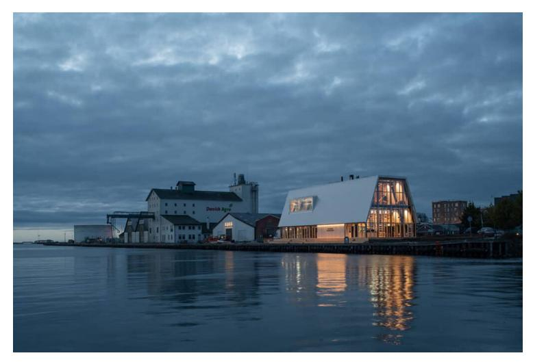
The building stands on a stretch of municipality-owned harbor quay that is considered a potential part of the city's climate adaptation strategy. To adapt to this possible temporary lifespan, the Braunstein Taphouse is "designed for disassembly" to make recycling the building components a realistic option if the building needs to be removed – either by relocating the entire building to a
