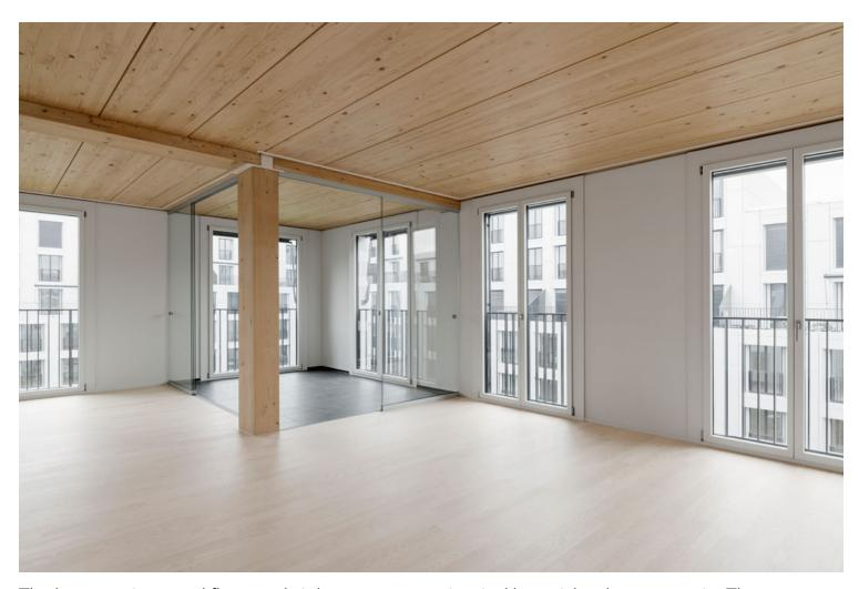
The basement, ground floor, and staircases are constructed in cast-in-place concrete. The remaining floors and exterior walls are built in wood. The façades use story-high windows of varying widths to subtly animate the building. By slanting the window reveals to the outside, the rooms behind are especially well lit. The floor-to-ceiling proportions resemble French balconies and allow the residents to step directly up to the façade.
