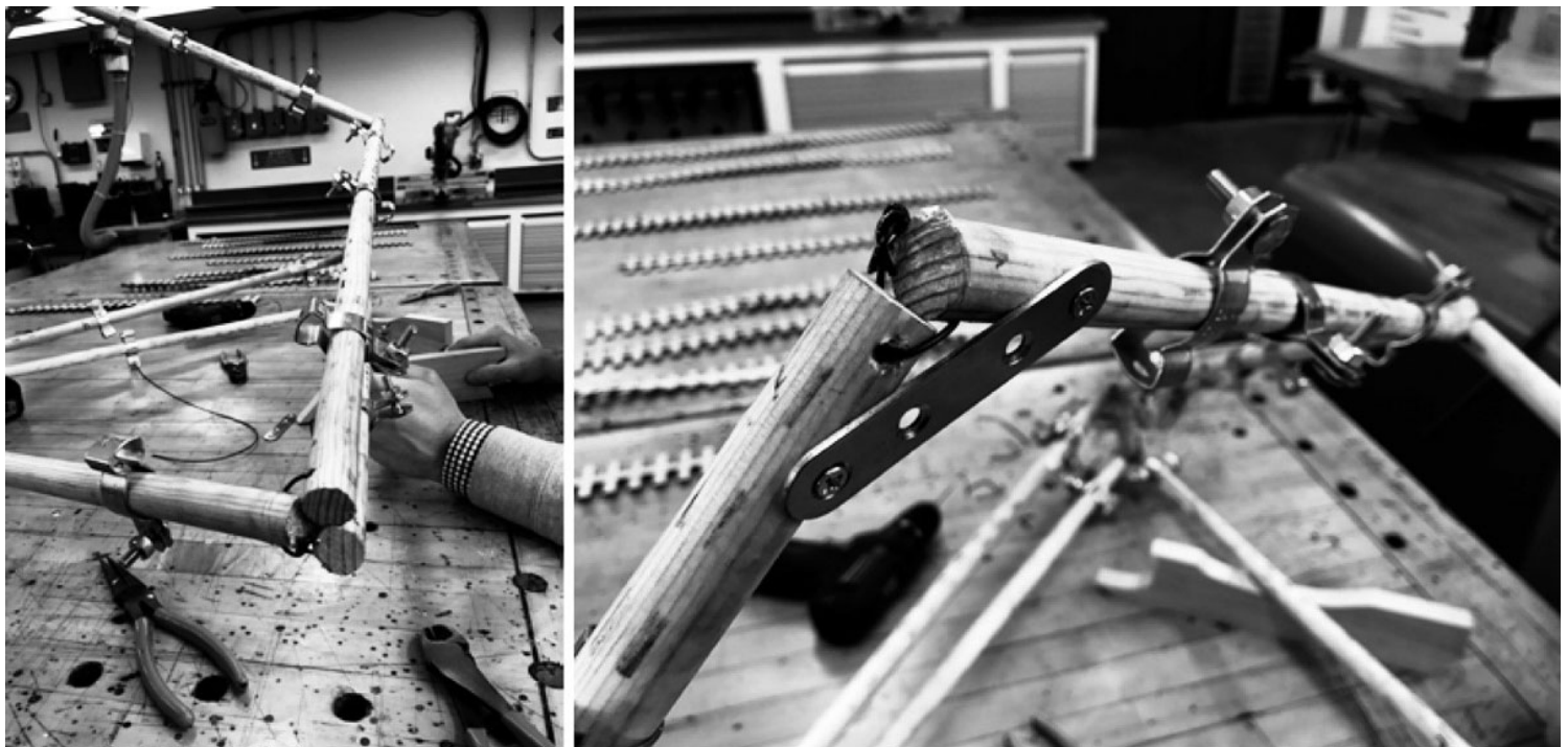
Figure 8. Galvanized steel conduits: telescoping members that are adjustable and removable, 2016.
