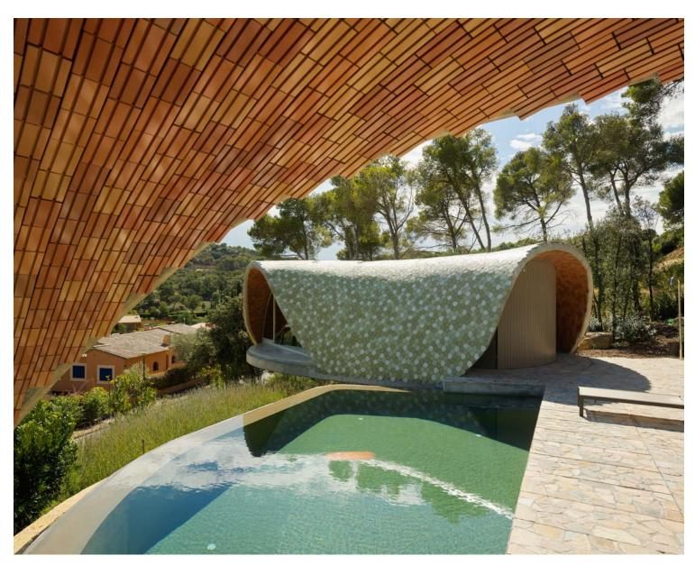
The exterior profile of the vault connects with the landscape, following the curves of the surrounding mountains. The green tones of the tiles outside blend in with the natural colors of the environment. For the interior, a special ceramic piece was designed to ensure optimum acoustic conditions.
