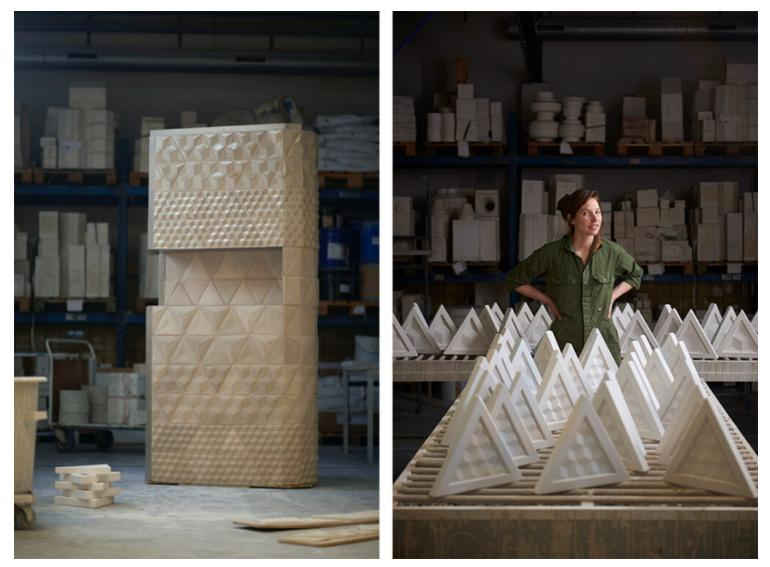
3D printed molds and the use of waste from other glazing processes.
