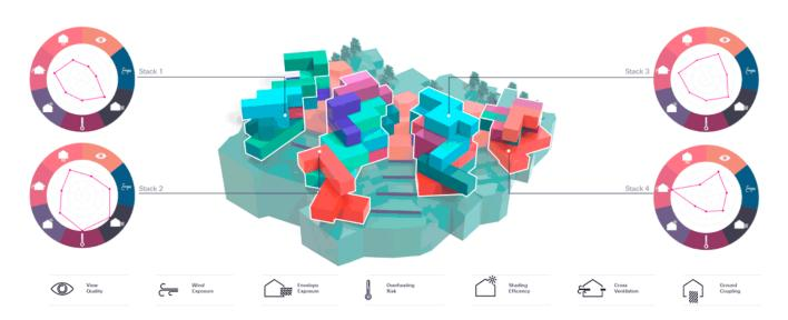
Hilson Moran developed the design's passive environmental control and water cycle strategies to minimize energy consumption by reducing temperatures to improve thermal comfort, with little or no requirements for mechanical ventilation. Dynamic thermal modelling was used to validate user comfort and energy consumption parameters.
