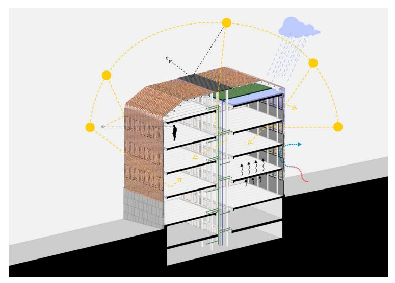
The construction systems are dry mounted (both the façade ceramics (Flexbrick) and the fiber cement partitions), avoiding supplementary railings and providing surfaces where the installations can be fixed (Euronit). The photocatalytic concrete base to the street helps filter the air of the city (Breinco), and the vegetal cover water tank collects rainwater for use in irrigation and toilets (Danosa).
