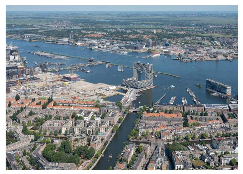
The building consists of a six floor low-rise block that wraps around a plaza on the waterfront. Two slender 60-metre-high towers at the open end of this block frame the river view. The towers carry a bridge spanning 48 metres, rising to a height of 90 metres above the city. The building is elevated 7
