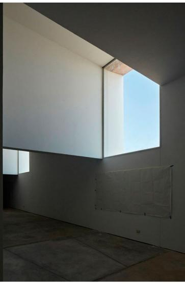
The building is constructed entirely with pozzolan cement, resistant to the desert's salty residue. The exposed concrete and polished cement that constitute its materiality acquire a natural reddish color that blends with the neighboring hills.
