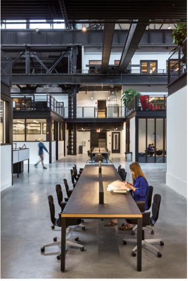
A second-story mezzanine is widened to accommodate additional rooms, connected by a steel grate catwalk lit underneath to mark the length of the building. The central axis, preserved as a simple circulation spine, exposes building-through views, a recall of the building's original factory floor layout.
