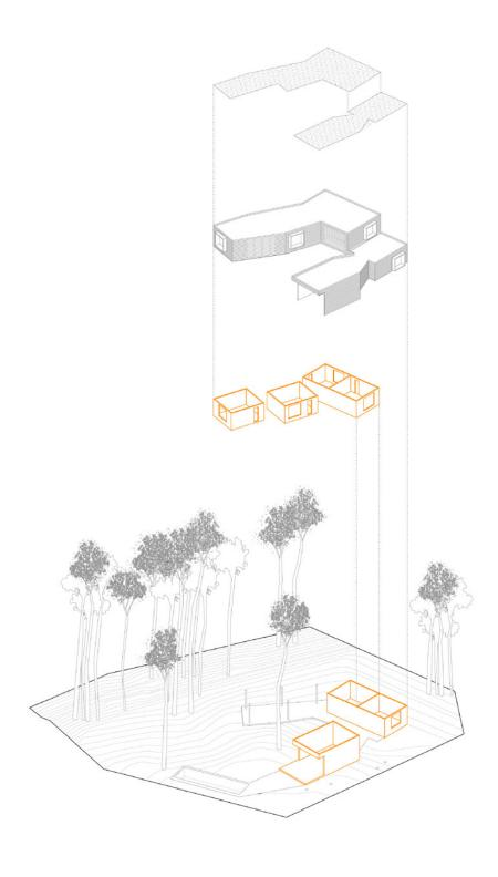
Concrete wooden-clad rooms Reinforced-Concrete, has a high thermal effusivity (2036 s<sup>1/2</sup> W/m<sup>2</sup> oC) and therefore has a high thermal storage capacity. On the other hand wood and projected cork have a low thermal effusivity (500 s<sup>1/2</sup> W/m<sup>2</sup> oC) and therefore are good insulator. The combination of both maximize energy storage, minimizing winter losses.
