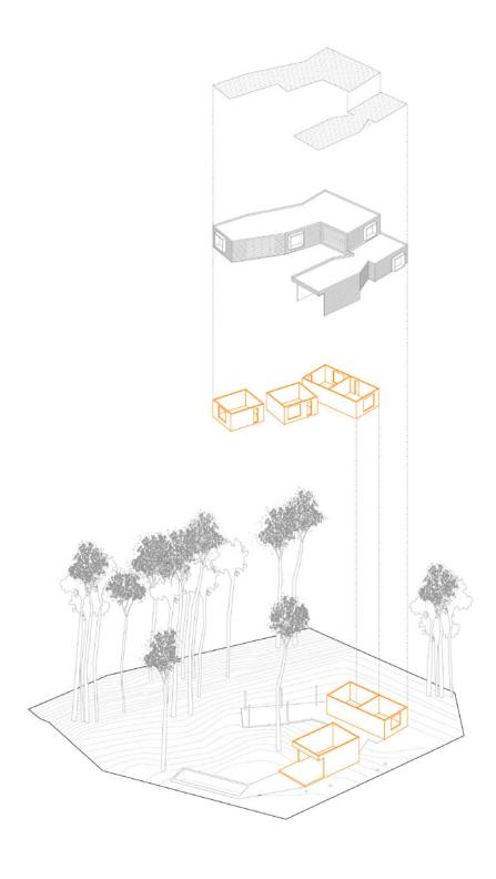
**Concrete wooden-clad rooms** Reinforced-Concrete, has a high thermal effusivity (2036  $s^{1/2}W/m^2$  oC) and therefore has a high thermal storage capacity. On the other hand wood and projected cork have a low thermal effusivity (500  $s^{1/2}W/m^2$  oC) and therefore are good insulator. The combination of both maximize energy storage, minimizing winter losses.
