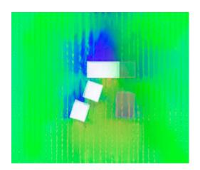
**Radiant rooms** Sun radiation penetrates the room through the window which, through direct radiation and greenhouse effect, heats-up the concrete floor and walls, storing energy. Insulation, through external wood cladding, prevents stored heat from dissipating. Combining window radiation collection with interior thermal storage and outdoor thermal insulation, the thermal performance of the room is enhanced.
