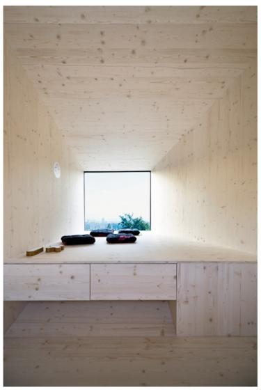
The prefabricated structure is made of timber frames, which are reinforced by plywood boards on both sides, encouraging low technology self-build possibilities. The thickness of the structural envelope is only 120mm including the structural joists and the plywood, mobilising every part of the surface as a structural stress skin and enabling a rigid system in the plane described by the ply.
