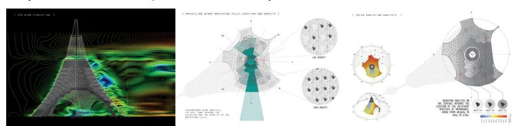
The system is able to be customized for the local context of hot and dry urban areas. Solar and wind analyses serve to define the position and the density, as well as the size of the cells.
