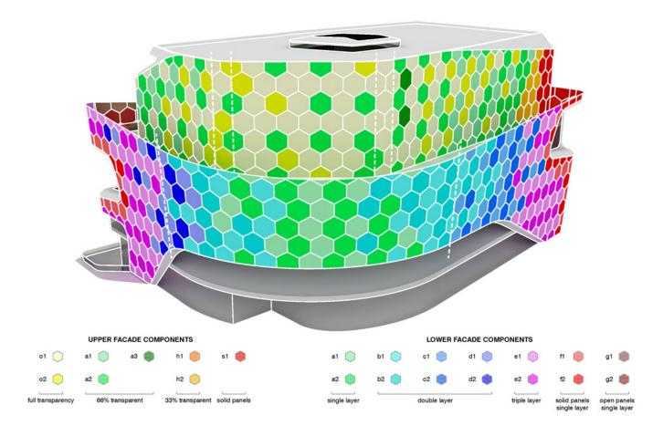
Based on a hexagonal grid, the façade components follow the articulated geometry of the building and provide constantly changing perspectives.
