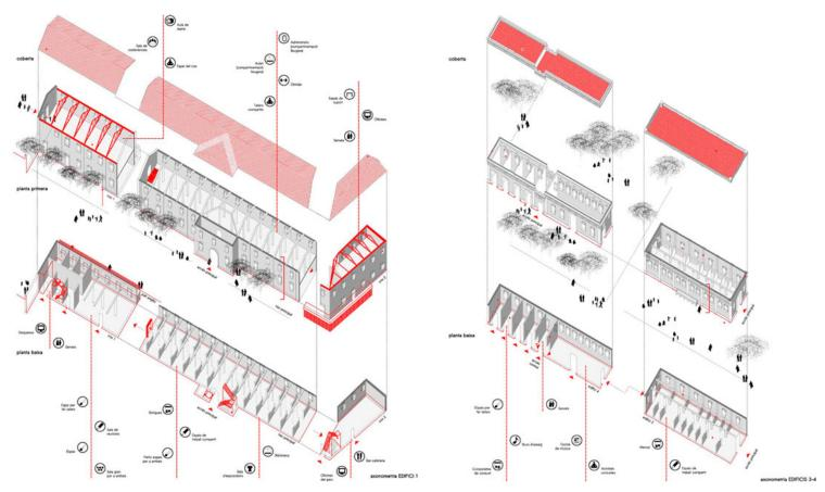
The original floors were maintained, as well as some old troughs and animal feeders, as an explanation of the building's initial function. Side entrances and service access points were created in the blind side façades. A window was also built into the upper corner of the first floor to avoid the appearance of a blind façade.
