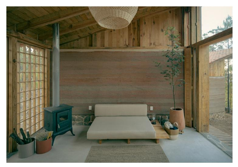
Waste management was incorporated into the design from the beginning. The house separates and filters grey and black water; it has rainwater collectors, a wood stove, solar panels, and gas. It uses passive strategies to reduce its energy consumption and takes advantage of the thermal qualities of the walls. The constructive knowledge of rammed earth walls was transmitted to the people of the nearby town, who participated in the work.
