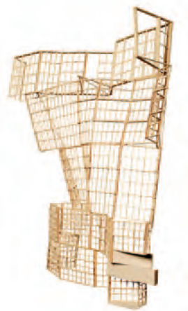
Balsa wood model of Miàs's Nowhere Skyscraper, study model for high-rise buildings.
