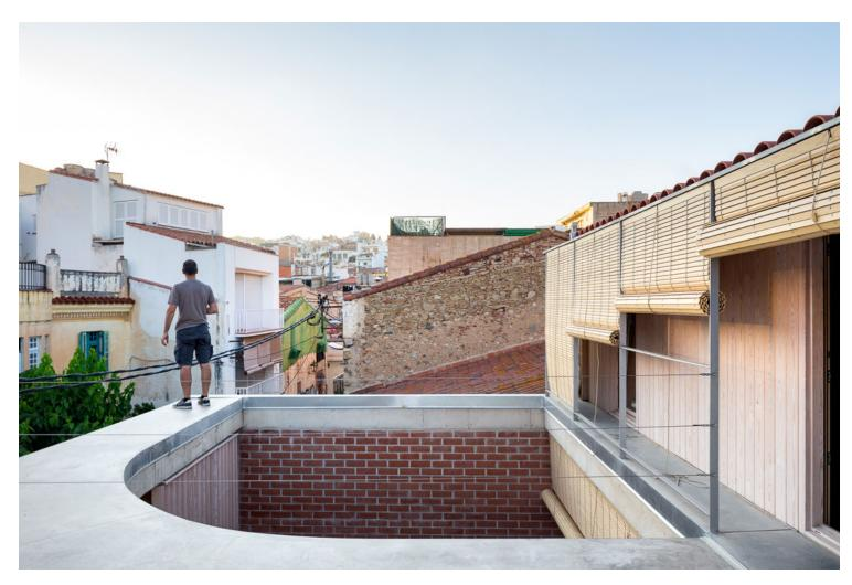
Heavy construction systems were chosen, such as concrete slabs and solid brick enclosures for their thermal insulation properties, all playing a key role in the building's desired passive performance. This inertia cushions and lags the daily and seasonal thermal oscillation and is especially suitable in a permanently occupied building: in this case, a home that also incorporates a workspace.
