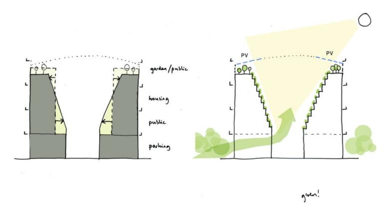
In the upper half of the Gasometer, housing will be built with an extensive mix of target groups and income classes – including a large proportion of social housing – to contribute to diversity. To provide these residences with sufficient daylight and outdoor space, without the effects of traffic noise from the adjacent motorway, the upper volume has been stepped out on the inside and provided with spacious galleries and terraces with abundant greenery. The gallery typology
