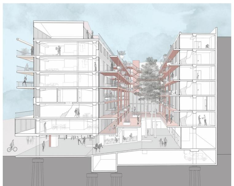
The 36-meter-deep parking garage will be opened up by creating a large courtyard while the upper floors will be partially deconstructed to form two parallel building volumes. The former central access ramp will be transformed into a generous and open threshold that marks the transition from
