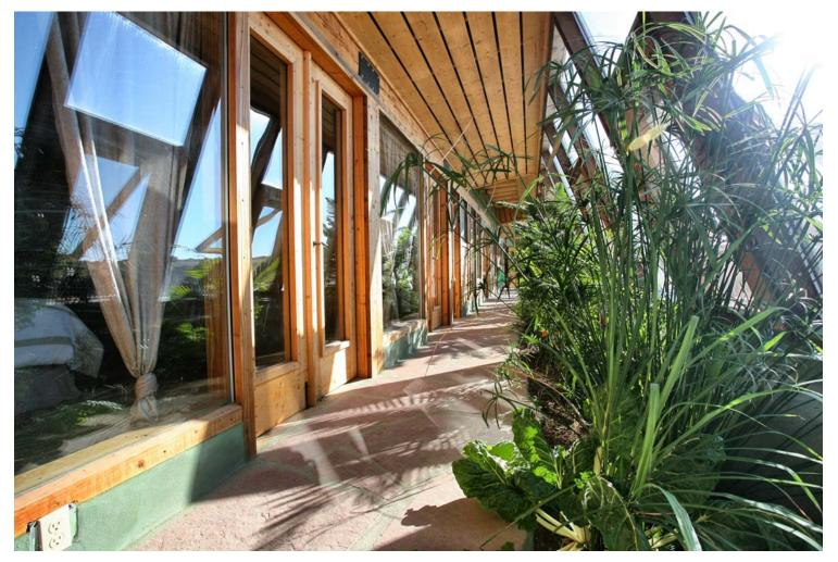
The <u>Global Earthship</u> design performs in almost any climate around the world. The main features of this design include a double layer of glass ("double greenhouse") between the inner living spaces and the outside and the use of underground cooling tubes and convection skylights which work together to provide ventilation and natural air conditioning for the building.
